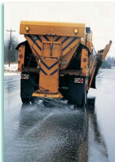
**FIGURE 14-10** The salts applied to icy roads are electrolytes. They lower the freezing point of water and melt the ice.
