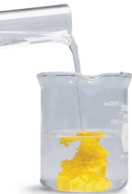
FIGURE 8-12 The double-replacement reaction between aqueous lead(II) nitrate, \text{Pb}(\text{NO}_3)_2(aq) , and aqueous potassium iodide, \text{KI}(aq) , yields the precipitate lead(II) iodide, \text{PbI}_2(s) .
