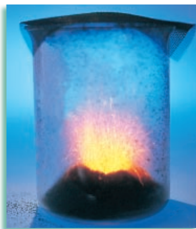
FIGURE 8-1 The decomposition of ammonium dichromate proceeds rapidly, releasing energy in the form of light and heat.
