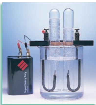
FIGURE 8-5 When an electric current is passed through water that has been made slightly conductive, the water molecules break down to yield hydrogen (in tube at right) and oxygen (in tube at left). Bubbles of each gas are evidence of the reaction. Note that twice as much hydrogen as oxygen is produced.
