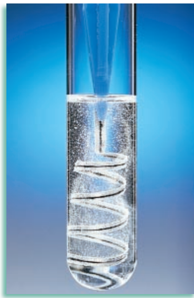
FIGURE 8-11 In this single-replacement reaction, the hydrogen in hydrochloric acid, \text{HCl} , is replaced by magnesium, \text{Mg} .
