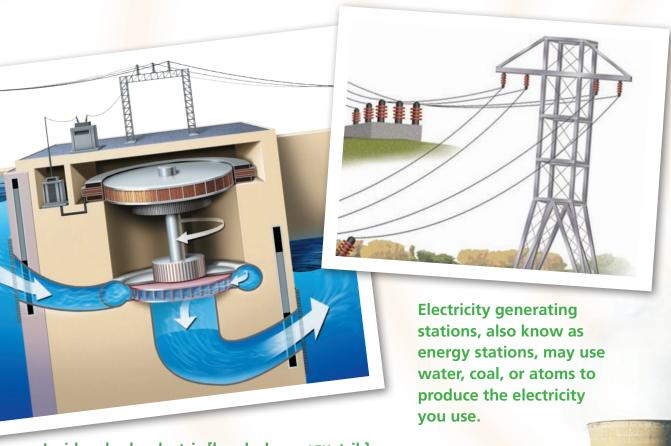
Inside a hydroelectric [hy•droh•ee•LEK•trik] dam, the mechanical energy of falling water is used to turn generators, which change mechanical energy into electrical energy.
