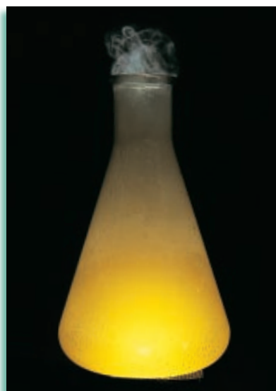
FIGURE 19-2 Sodium and chlorine react violently to form NaCl. The synthesis of NaCl from its elements illustrates the oxidation-reduction process.
