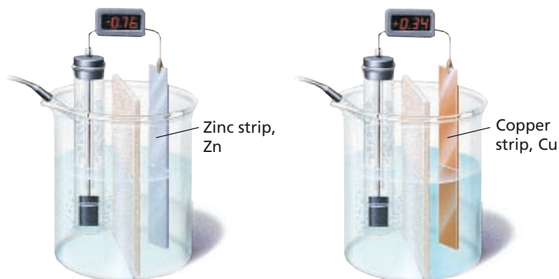
FIGURE 19-18 The electrode potentials of zinc and copper half-cells are measured by coupling them with a standard hydrogen electrode.
