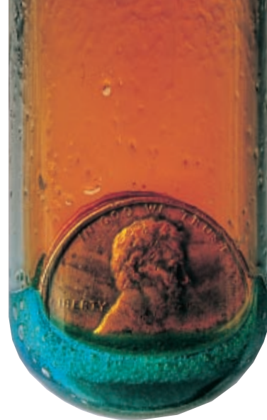
FIGURE 19-3 Copper is oxidized and nitrogen monoxide is produced when this penny is placed in a nitric acid solution.
