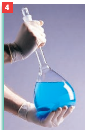
FIGURE 13-17 The preparation of a 0.5000 M solution of \text{CuSO}_4 \cdot 5\text{H}_2\text{O} starts with calculating the mass of solute needed.
