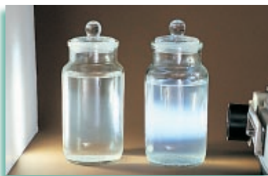
FIGURE 13-4 A beam of light distinguishes a colloid from a solution. The particles in a colloid will scatter light, making the beam visible. The mixture of gelatin and water in the jar on the right is a colloid. The mixture of water and sodium chloride in the jar on the left is a true solution.
