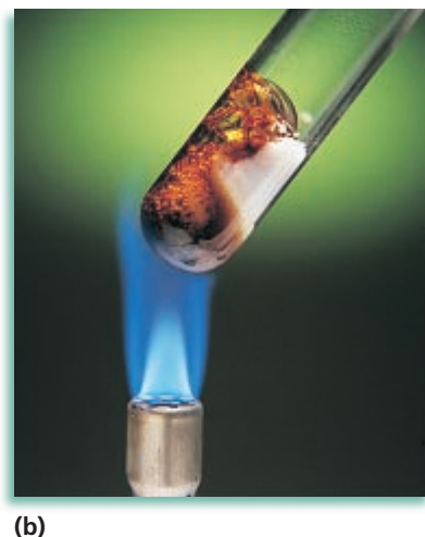
FIGURE 1-10 (a) Passing an electric current through water causes the compound to break down into the elements hydrogen and oxygen, which differ in composition from water. (b) When sucrose is heated, it caramelizes. When it is heated to a high temperature, it breaks down completely into carbon and water.
