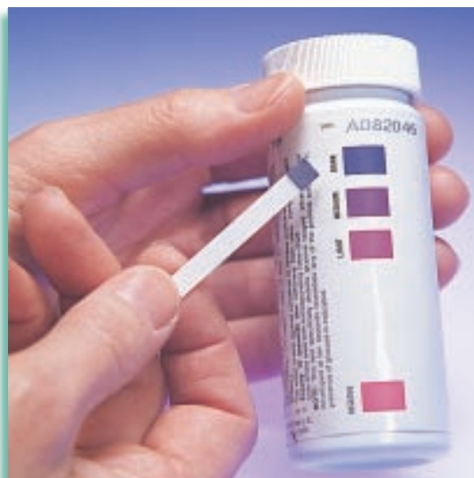
FIGURE 1-4 Because it possesses certain chemical properties, a test strip containing Benedict's solution is used to test for the presence of sugar in urine. The test strip is dipped into the sample. The test strip is then matched to a color scale to determine the sugar level in the urine.
