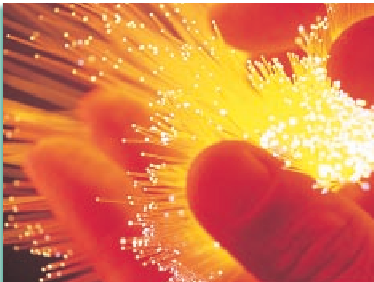
FIGURE 1-2 The chemical structure of the material in an optical fiber gives it the property of total internal reflection. This property, which allows these fibers to carry light, was discovered through basic and applied research. The use of this property to build telecommunications networks by sending data on light pulses is the technological development of fiber optics.
