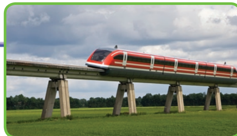
▲ Maglev trains use magnets to lift them above the tracks while moving.
